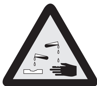
Danger by acid media! Protective equipment necessary!
